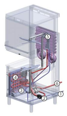
The Steam Heat Recovery (SHR) device (patented) recovers and condenses the steam that forms during the rinsing cycle and uses it to raise the intake water temperature by 10°C. The result is that the working environment is healthier and more comfortable and energy consumption is reduced.
